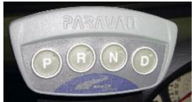
Electronic gear selector, from Adaptacar
