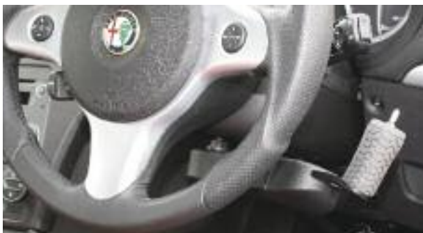
Jeff Gosling single lever accelerator and brake – here fitted with optional indicator switch
