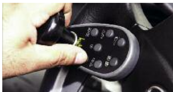
Steering knob combined with wireless secondary controls, from Autoadapt
