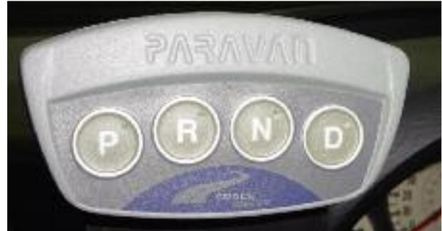
Electronic gear selector, from Adaptacar
