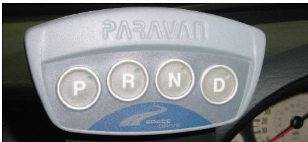
Electronic gear selector – Adaptacar
