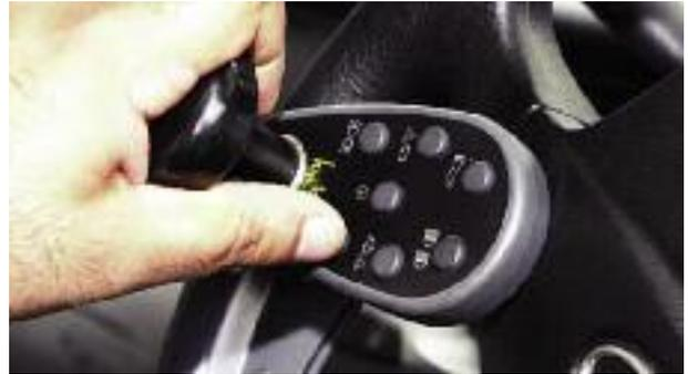
Steering knob combined with wireless secondary controls
