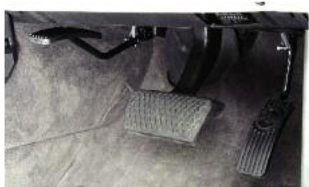
Flip up pedal – here the right pedal is down
