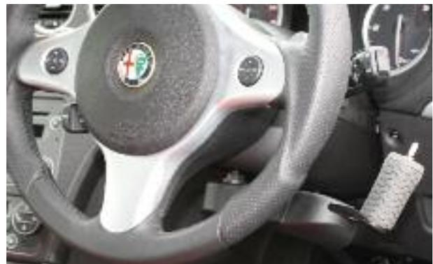
Single lever accelerator and brake – here fitted with optional indicator switch
