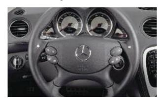
Gear controls on steering wheel
