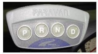
Electronic gear selector, from Adaptacar
