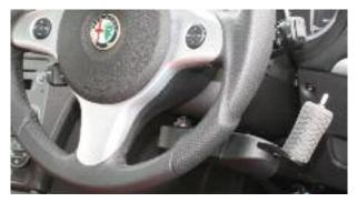
Jeff Gosling single lever accelerator and brake – here fitted with optional indicator switch
