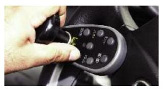
Steering knob combined with wireless secondary controls, from Autoadapt
