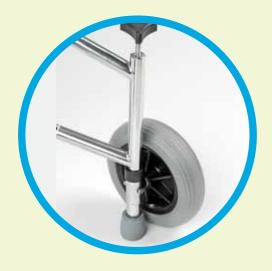
Pressure brakes go on when you push down on the frame (see picture - above). They are easy to use because it is easy to use your weight to press down. They only stay on while you are pushing, so you cannot lock the brakes on if you want to stay put for a while. Make sure they are properly adjusted, otherwise they might come on when you are not expecting it.
