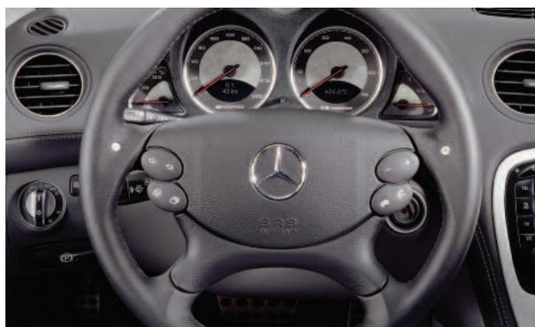
Gear controls on steering wheel
