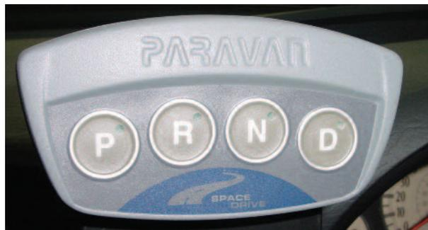
Electronic gear selector, from Adaptacar
