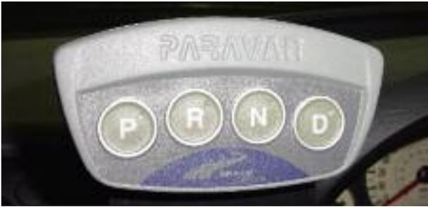
Electronic gear selector, from Adaptacar
