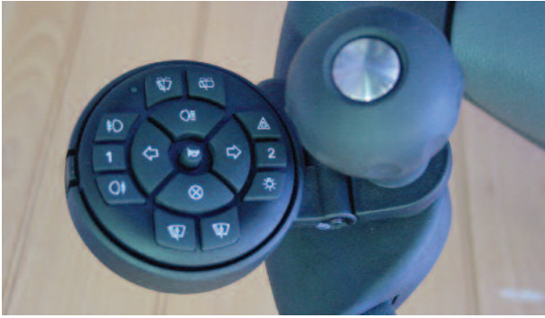
Steering knob combined with wireless secondary controls – Lodgesons
